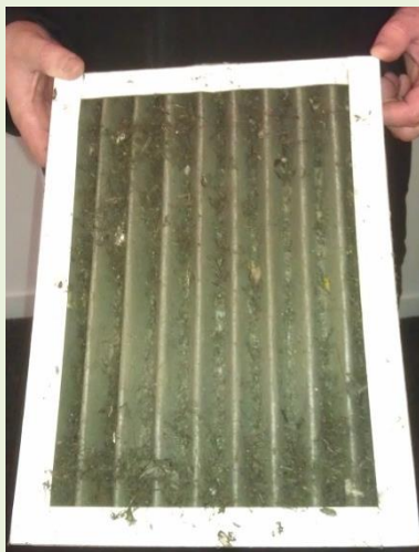
Figure 12: Insects blocking the MVHR filter
