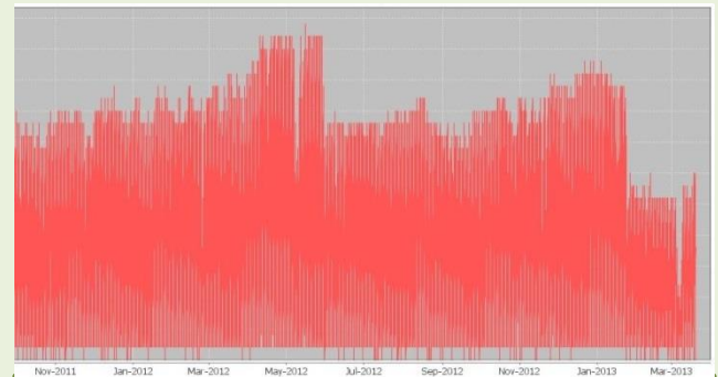
Figure 24: Daily MVHR electricity consumption
